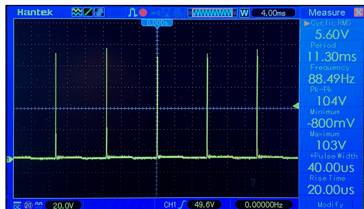
Fig 34: HV pulses with a 10:1 potential divider
