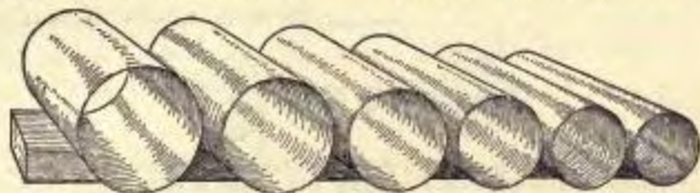
FIG. 60.—Lodge's Electric Retina—a set of copper cylinders 40 centims. long, and of diameters 14, 13, 12, 11, 10, 9 centims.; facing a source of radiation, as do the rods and cones in the eye, and responding by diametral electric vibration to the appropriate frequency. Nature , vol. 41, p. 462; cf. also p. 258 above.
