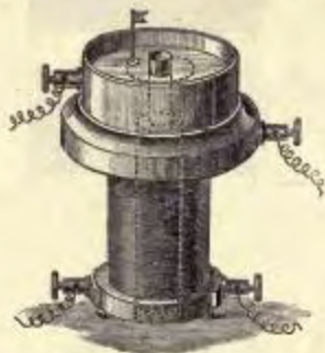
Fig. 22.—Rotation of a liquid disk conveying a radial current in a vertical magnetic field.
