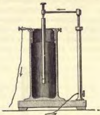
Fig. 26.—Another mode of exhibiting the same thing as Fig. 25. The magnet is loaded so as to float upright in mercury.
