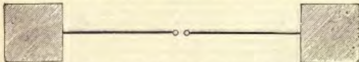
FIG. 63.—Gigantic oscillator, drawn to scale \frac{1}{100} , for violent and distant effects. When this is excited by very large coil, most gas and water pipes in the building, and some wire fencing also, give off sparks to conductors brought close to them or to each other; and a telephone joined to any conductors in the neighbourhood is affected. See Lodge, on "Signalling across Space without Wires" (Electrician Co.) Rate of vibration, 10 million per second. Average radiation activity, while it lasts, 64 horse-power.
