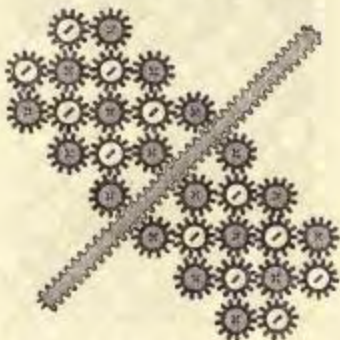
FIG. 30.—A provisional representation of a current surrounded by dielectric medium, either propelling or being propelled. Section through the wire. Compare Fig. 30, b .
