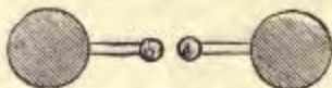
FIG. 62.—Small oscillator, drawn to scale \frac{1}{4} , used for experiments with the pitch lens. (Lodge and Howard, Phil. Mag. , July 1889. Rate of vibration, 300 million per second.
