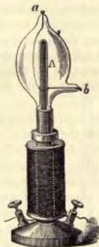
Fig. 24.—Induction coil discharge from a to b through rarefied gas, rotating round a glass protected magnetized iron rod.
