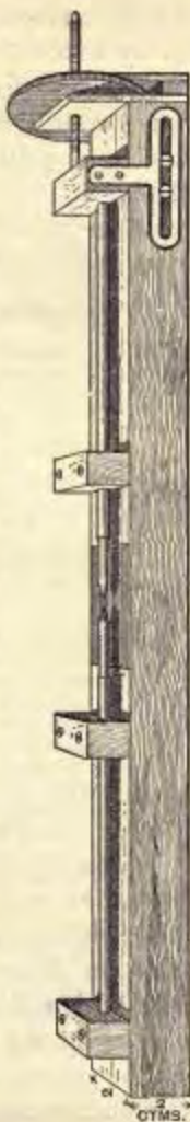
FIG. 58.—Linear receiver used by Lodge. A pair of copper wires each 56 centims. long, held in glass tubes a trifle shorter, and one of them movable by a screw with large head. Mounted on teak board 60 x 2 centims.
