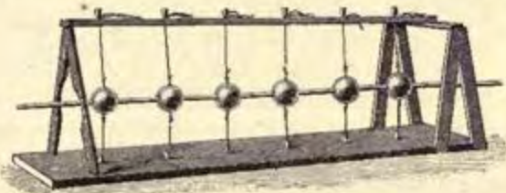
FIG. 8.—Partial model of a dielectric.
