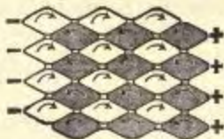
FIG. 46.—A portion of an electrostatic field between two oppositely charged bodies with its lines of force going from right to left, and showing a tension along and a pressure at right angles to them, due to the elasticity of the cells (which elasticity may be due to their containing fluid in a state of whirl, see § 125). Magnetic lines of force perpendicular to the paper are also shown in section. While this magnetic field was being excited and propagated from below upwards, a slight strain would be produced in the elastic cells, like but immensely less than that shown; as contrasted with its normal condition (Fig. 37). Conversely, while this electrostatic strain was being produced, the positive whirls would be infinitesimally quickened and the negative ones retarded during the displacement, thus producing a minute magnetic effect. If the medium is not magnetized, the whirls are not necessarily absent, only faced all ways.
