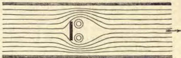
FIG. 14.—Stream-lines of water flowing through a pipe with an obstruction in it.
