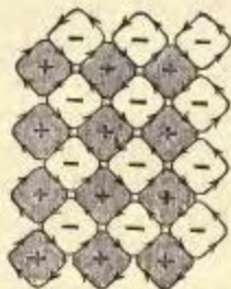
FIG. 37.—Section of a magnetic field perpendicular to the lines of force. Alternate cells rotating oppositely. Another mode of drawing Fig. 36.
