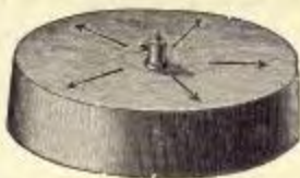
Fig. 19.—Another pivoted disk with flange to dip into liquid so as to make contact all round its rim. It rotates when a magnet is brought above or below; or even in the field of the earth.
