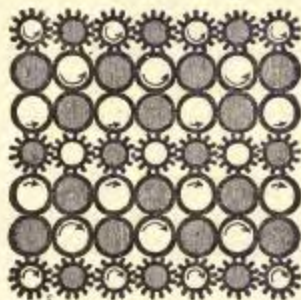
FIG. 44.—Two parallel conductors conveying equal currents in one direction and getting pushed together by the centrifugal force of the outside whirls, no whirl existing between them. The length of the arrows again suggests the distribution of magnetism in the conductors. Fig. 40 showed the correlative repulsion of opposite currents.
