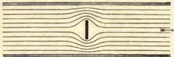
FIG. 15.—Electrical stream-lines past an obstacle.
