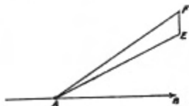
FIG. 16.—A is the charge, AB its line of motion, and AE its electric force in a certain direction when stationary; EF is the magnetically induced electric component due to the motion and AF is the resultant electric force which replaces the original force AE. The magnetic force, to the motion of which EF is due, is perpendicular to the paper, and is itself caused by the motion; hence KF is a quantity of the second order and is small for speeds distinctly less than that of light.
