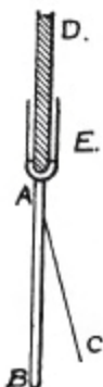
FIG. 24.—Working part of the above electroSCOPE, magnified four times. The rod AB with the gold leaf C is cemented to a thin rod of melted quartz D by means of a drop of mastic or guttapercha at the bottom of a minute metallic capsule E attached to the rod AB; thereby lessening any tendency of the charge to creep, and keeping the capacity exceedingly small.
